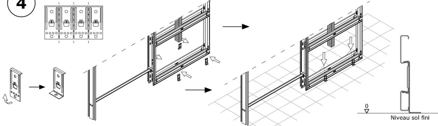
**SOLUTION 2** (INSÉRER LE CHÂSSIS ENTRE DEUX CORNIÈRES MÉTALLIQUES COLLÉES AU SOL)
