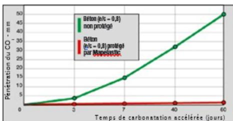
FIG. 2 : EFFET DU MAPELASTIC SUR LA CARBONATATION ACCÉLÉRÉE (30% DE CO<sub>2</sub>) D'UN BÉTON POREUX
